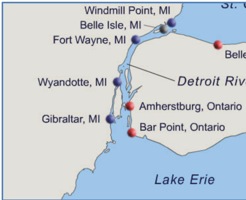
Figure 51. Locations of U.S. (blue), Canadian (red), and USACE (gray) water level stations on the Detroit River ( http://www.great-lakes.net/envt/water/levels/levels_current.html ).
