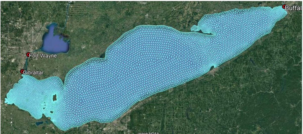
Figure 1. The upgraded LEOFS model grid and the location of stations that provide boundary conditions.
